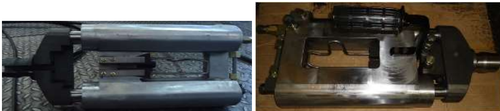
Fig: Assembly of Twin Ram Single pull Hydraulic Jack
